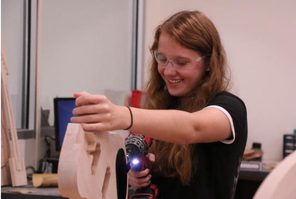
Maddie Weldon, 16, drills a hole for an input jack on the bottom of her guitar.
